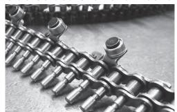
In order to maintain support of an offset pusher attachment rollers are fitted to standard 'K1' attachments, which run in tracks alongside the chain. The chain has special extended pins on every pitch to allow change in positions of the pushers to accommodate different sizes of packaging. Cross+Morse have produced many special pusher plates for packaging machines, which can be supplied assembled in the chain, or as individual links for customers to fit to their own chains.
